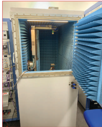
▲ Fig. 4 Anechoic chamber with spherical scanner, measurement probe supported by the elevation arm, and DUT positioned at the azimuth pole.
